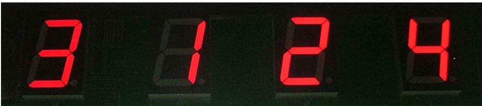
Figure 4. When each car passes the finish line, its finish position is displayed on the LED.
