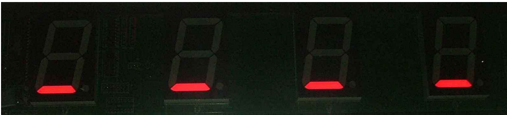
Figure 3. When the Start Gate is opened, the dash moves to the bottom of the LED display indicating that the race is on.
