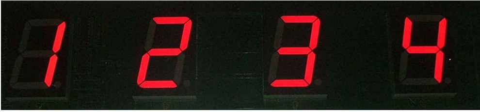
Figure 1. When the Timer is first powered up, the display shows the lane numbers from left to right. The message shown in Figure 5 is also sent to the serial link at this time.
